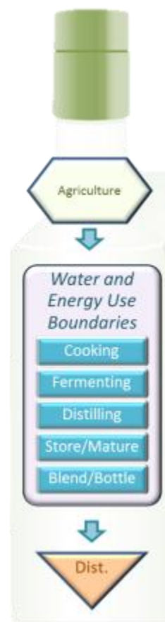
Figure 12: Process Map, Distillery
