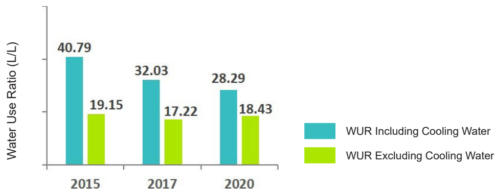
Figure 12: Effect of Cooling Water on Water Efficiency, 2015-2020
